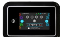
in.k1000 main keypad Color LCD capacitive touchscreen display
