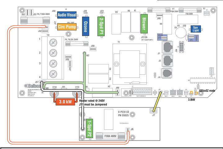
**WARNING:** Main Power to system should be turned OFF BEFORE adjusting DIP switches. **WARNING:** Persistent Memory (J43) must be RESET to allow new DIP switch settings to take effect. (See Persistent Memory page)
