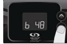
The values displayed by the system correspond to 80% of the maximum amperage capacity of the GFCI.
