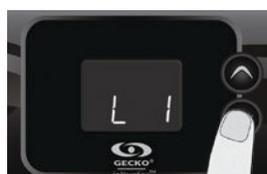
When starting up, the control system will download the different low-level configurations from the in.stik's memory. The low-level selection menu will then appear.
